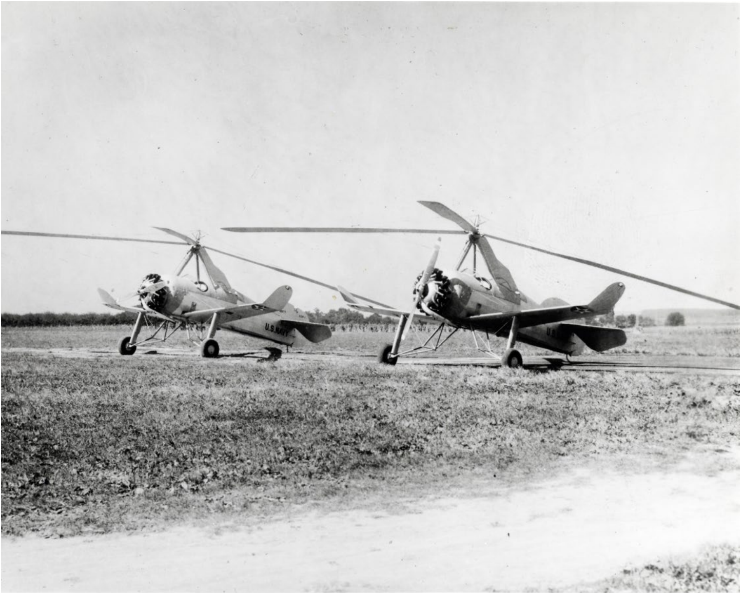
[Photo 3 – A pair of US Army Air Corps Pitcairn PCA-3 Autogiros. Credit: National Museum of the US Air Force]
